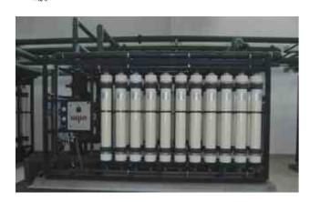
adopting new membrane separation technology, MC-CL ultrafiltration water purification equipment is widely used in various drinking water, mineral water, beverage and water for food industry; water for aquatic product processing; clarification and bacteria removal in wine as well as medicine production; pretreatment or terminal treatment of pure and ultrapure water production for electronic industry; recycling of industrial wastewater and useful substances; water for power plant, etc.
