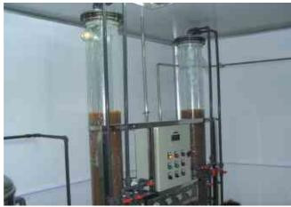
MC-JYH anion and cation mixing exchanger is a kind of ion exchange device in which anion and cation exchange resin is filled layer by layer in the same column according to a certain proportion. The anion resin and cation resin is closely and staggeredly arranged in the evenly mixed resin layer. Each pair of anion resin and cation resin particle is similar to a combined bed, so the mixed bed can be regarded as an ion exchange equipment with numerous combined beds running in series.
