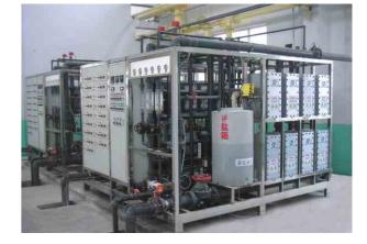
EDI (Electro-deionization, continuous Electrode ionization) uses mixed ion exchange resin to adsorb the anion and cation ions in the feed water. Meantime, under direct
